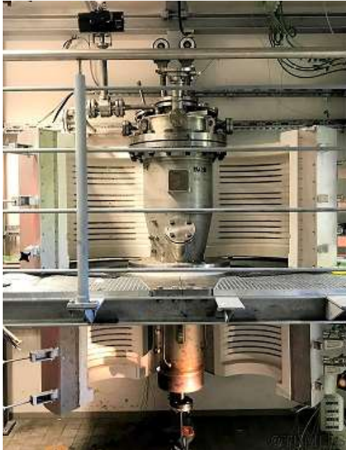
Fluidized bed reactor with 30 litre volume (700 degrees Celsius, 6 bar) Photo credit: TUMLES (Technical University of Munich/Chair of Energy Systems) Download: https://drive.google.com/file/d/1o4yQqTuFjeA2JVXMZVc8mVeRjdvUKYYc/view?usp=sharing
