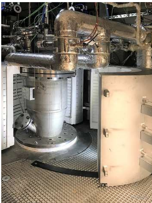
Fluidized bed reactor with 30 litre volume (700 degrees Celsius, 6 bar) Photo credit: TUMLES (Technical University of Munich/Chair of Energy Systems) Download: https://drive.google.com/file/d/1-2TPaklmah2z6Q9DIM-VP9ZFStDpMRdv/view?usp=sharing
