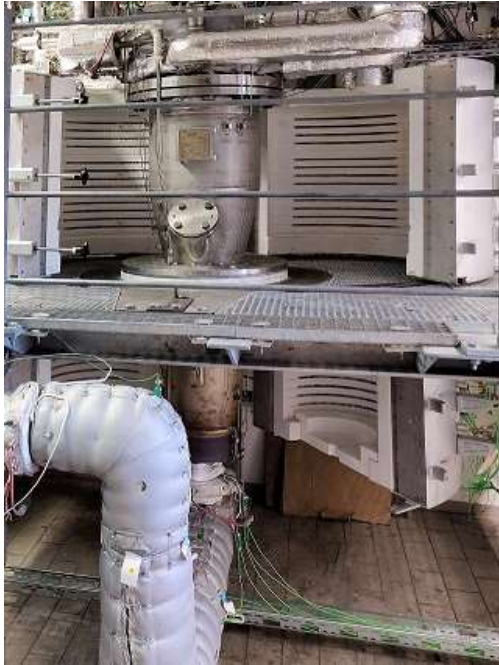
Fluidized bed reactor with 30 litre volume (700 degrees Celsius, 6 bar)
